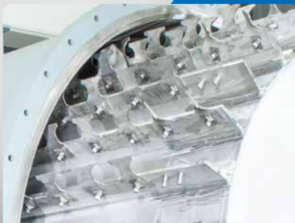
Rotor blades sewage sludge drying
