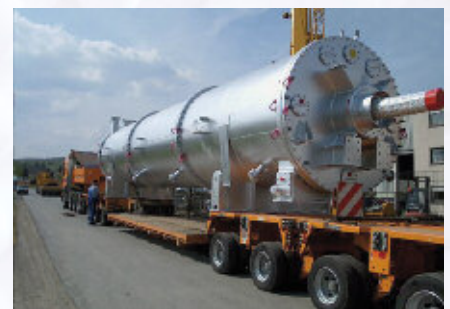
Transport of sludge dryer
