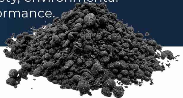
Figure 1: Fully dried sludge 90% dry solid
